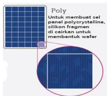
Gambar 4. Panel surya jenis polycrystalline
