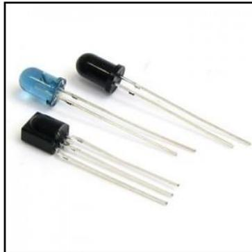
**Gambar 2.8** Led infrared
