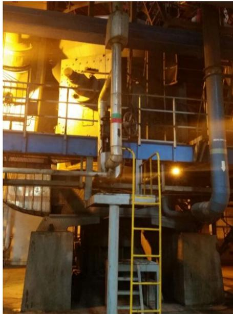
Gambar : 2.4 Mill/pulverized
