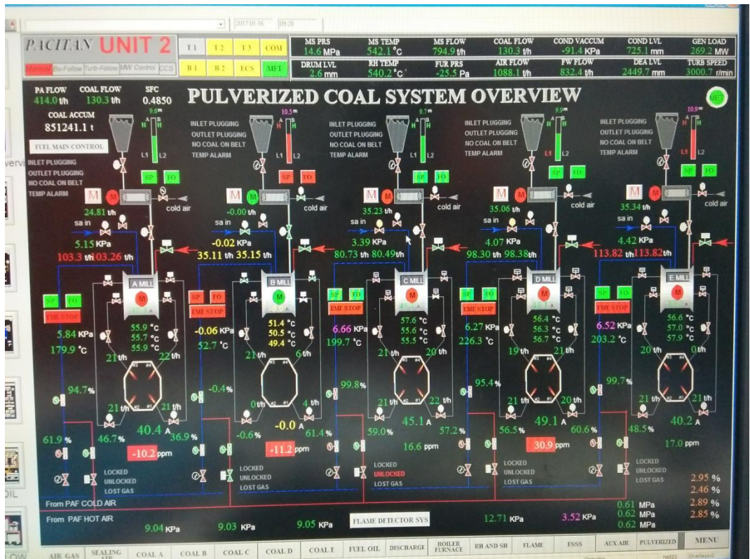
Gambar : 5.3 Distributed control system (DCS) pulverized coal system
