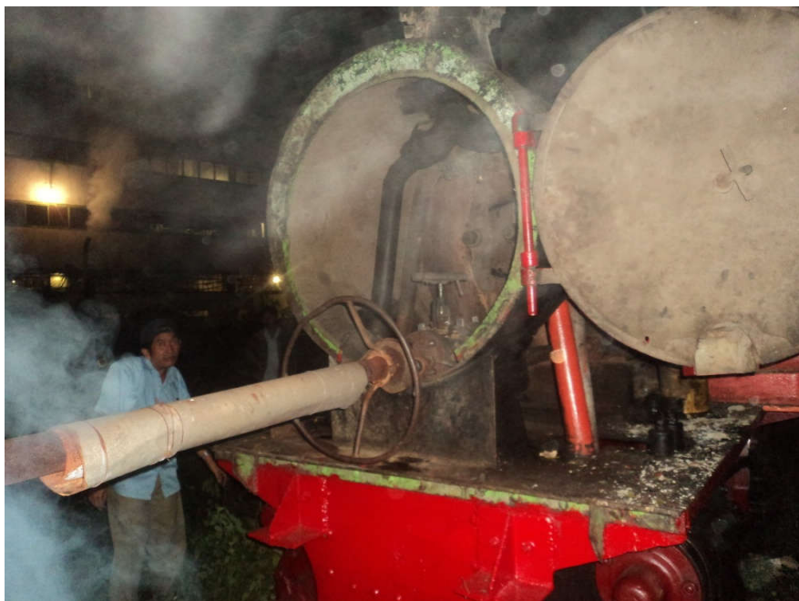
PROSES STEAM CHARGING
