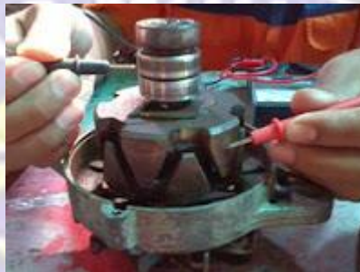
Hubungan massa rotor coil
