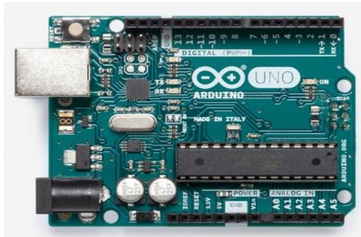
Gambar 2.4 Bord Arduino Uno
