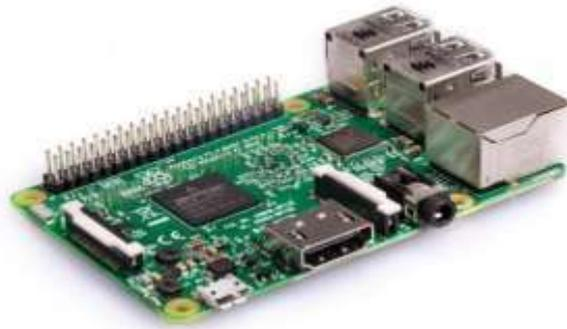
Gambar. 2.1 Raspberry pi 3 model B
