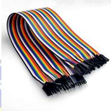
Gambar 2.7 Kabel Jumper
