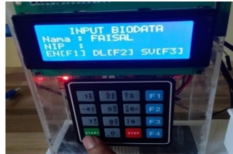
Gambar 9 Hasil Input Biodata User Melalui Keypad
