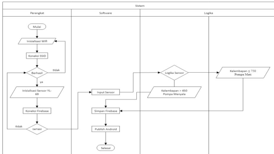
Gambar 3. Flowchart sistem *integrated device electronic*
