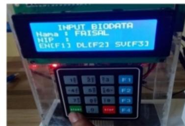
Gambar 9 Hasil Input Biodata User Melalui Keypad
