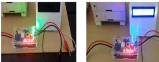
Gambar 5 Pengujian Power Supply Arduino
