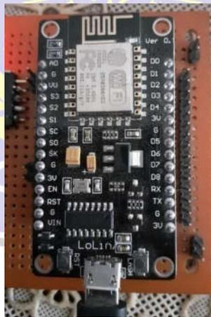
Gambar 2.1 Module *NodeMcu*
