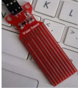
Gambar 2.5 Sensor *Water Level*
