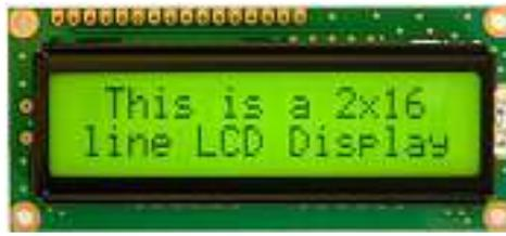
**Gambar 2.6** LCD 16 X 2
