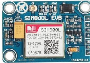
Gambar 2.9 Modul GSM Sim800L V2
