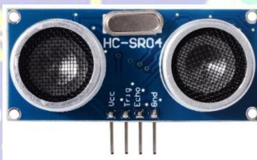
Gambar 2.4 Sensor Ultrasonik HC-SR04
