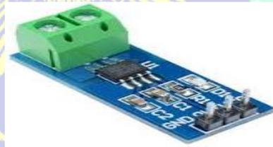
Gambar 2.8 Modul Sensor Arus ACS712
