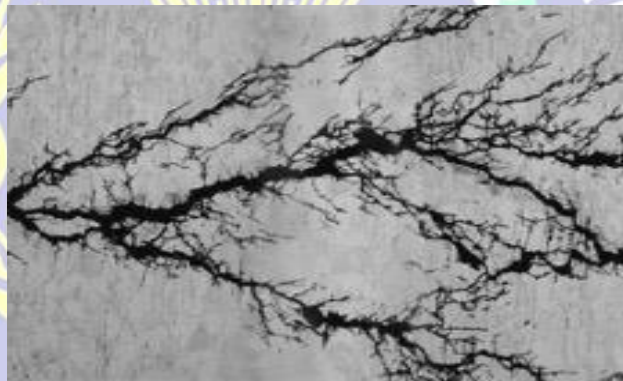
Gambar 2.11 Stress Corrosion Cracking (Corrosionclinic, 2013)
