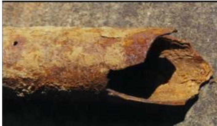
Gambar 2.3 Korosi Merata ( Corrosionclinic , 2013)
