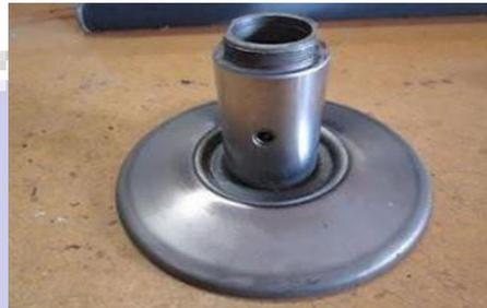
**Gambar 2.15 Puli Bergerak (sliding sheave). (Otosigna99)**
