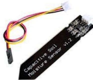
Gambar 2.2.5 Soil Moisture Sensor
