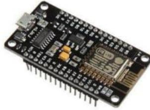
Gambar 2.2.4 NodeMCU ESP8266
