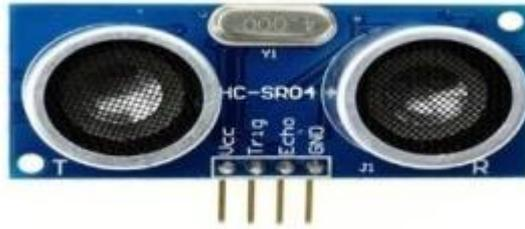
**Gambar 2.1** Sensor Ultrasonik
