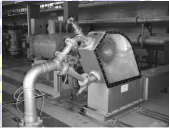
Gambar 2.18 Rumah Turbin Pelton Skala Laboratorium (Suyesh, 2019)
