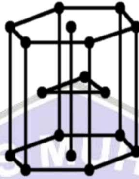
Gambar 2. 4 Konfigurasi struktur kristal hexagonal close-packed
