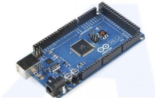
Gambar 2. 11 Arduino Mega 2560
