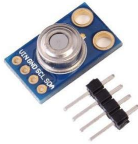
Gambar 2.2 Sensor Suhu GY-906 MLX90614
