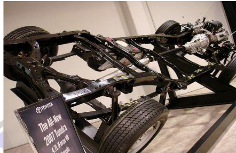
Gambar 2.3.0 Ladder Frame Chassis
