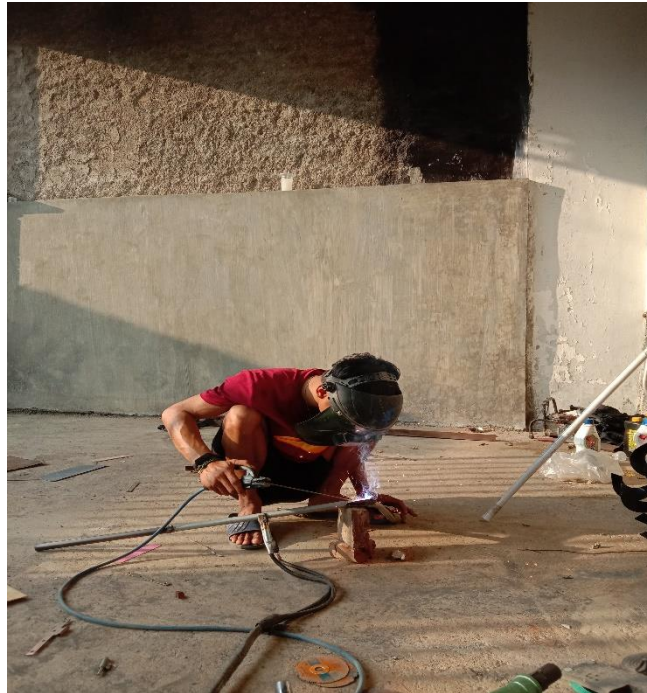
Proses Pengelasan Kerangka Tractor Portable
