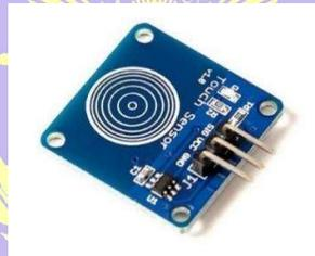
Gambar 2. 7 *Capacitive Touch Sensor*
