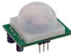
Gambar 2. 4 Sensor PIR (*Passive InfraRed*)
