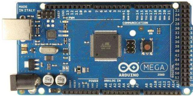
Gambar 2. 9 Arduino Mega 2560
