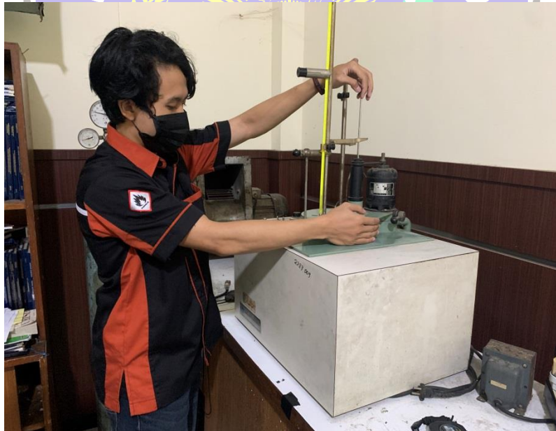
Pengujian nilai kalor (Bomb Calorimeter)
