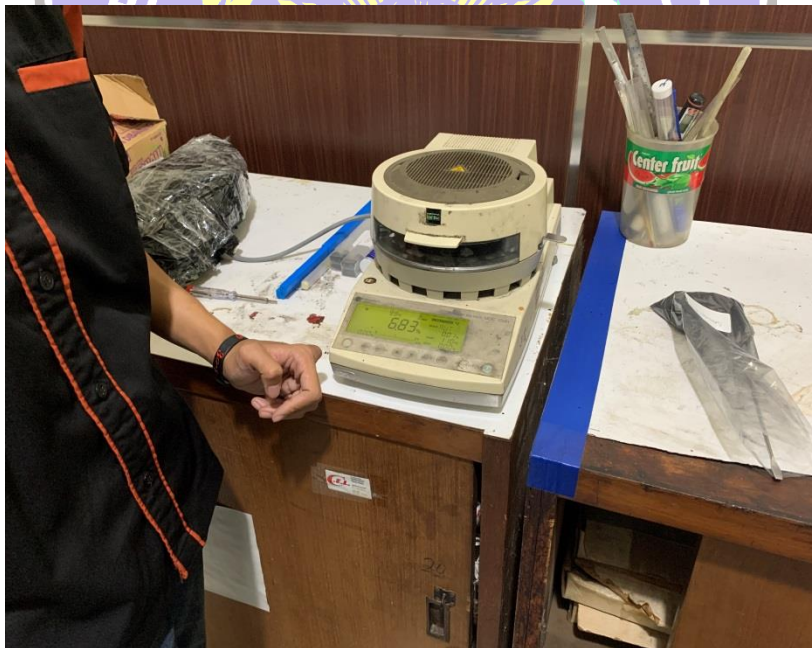
Pengujian kadar air (Moisture Analyzer)
