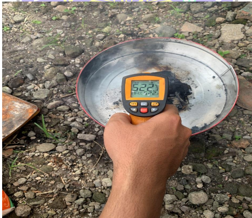
Pengukuran temperature Briket
