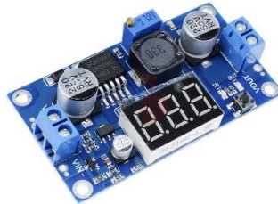
Gambar 2.13 Step Down Tegangan Dc LM2596S
