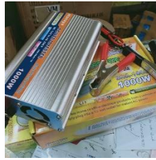
Gambar 2.4 Inverter DC to AC
